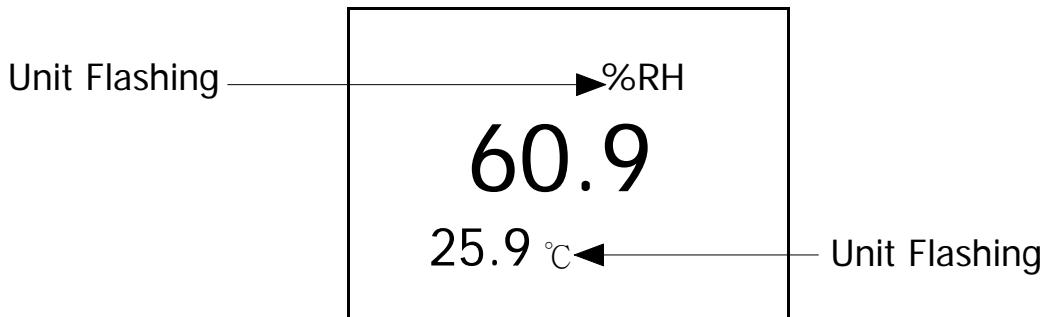
***The measuring unit for different mode***
